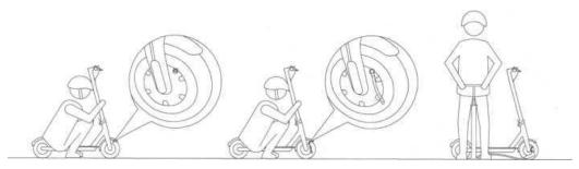
If your electric scooter front and rear tires are deficency, please use the extended inflatable mouth to connect the scooter body tires to cheer. First remove the front and rear tire inflatable mouth cup, and then tighten the extension of the inflatable mouth and tire inflatable mouth, and connect the pump to inflate after they are to be tightened
