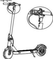
3. Use the hex wrench in the packing box to lock screws on both sides.
