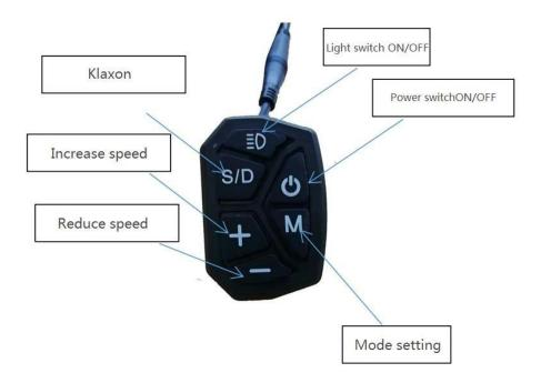
Power ON/OFF button: Long press 3S to power on. Long press 3S to power off.
