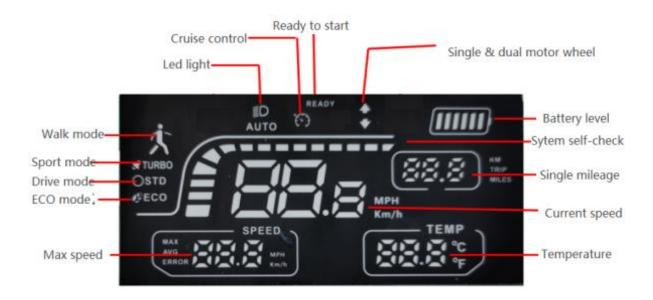
Power display: Six led lights on the display show battery power.
