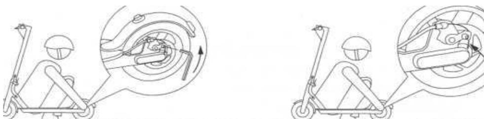
If you feel the brakes are too tight, please use the M5 hex wrench counterclockwise to release the pressure plate screws on the disc brake seat, return the brake line to make the exposed tail length slightly shorter, and lock the pressure plate screws; If you feel the brake is too loose, release the
