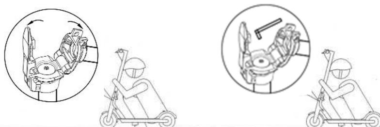
If your standpipe in electric scooter is shaking, please use the M5 hex wrench to lock the two screws at the fold mechanism.
