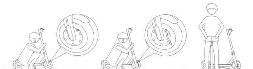
If your electric scooter front and rear tires are deficiency, please use the extended inflatable mouth to connect the scooter body tires to cheer. First remove the front and rear tire inflatable mouth cup, and then tighten the extension of the inflatable mouth and tire inflatable mouth, and connect the pump to inflate after they are to be tightened
